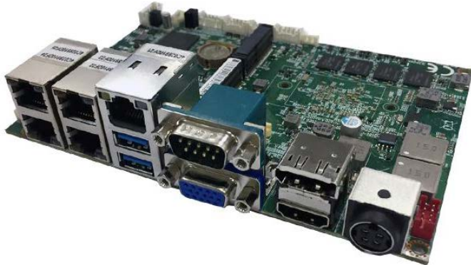
Figure 1. The LEX Computech 3I390NX Series motherboard provides four PoE ports. (Source: LEX Computech)
